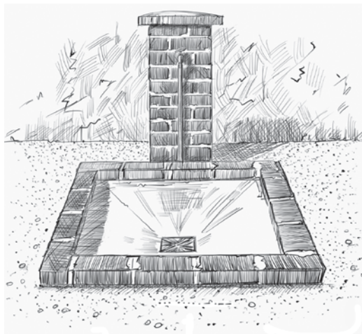
Figure 12.2 Simple sluice for disposal of faeces
