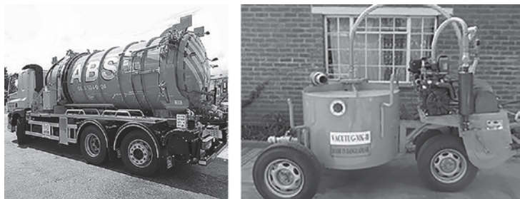
Typical commercial vacuum tanker Small vacuum tanker for high-density housing areas
