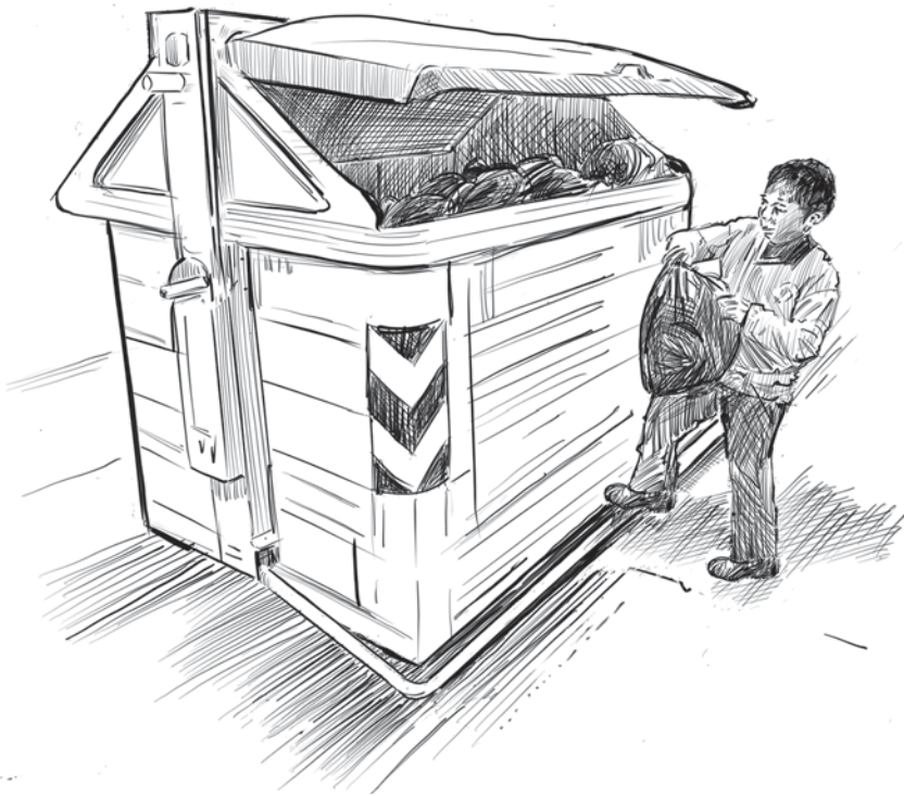
Figure 15.2 Foot-operated solid waste storage container suitable for mechanized emptying
